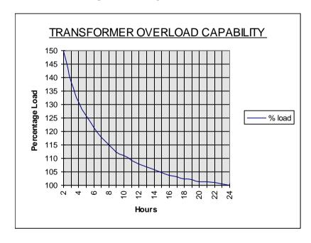
The maximum load at other periods is assumed to be 70% of the transformer rating for the above transformer overload capability curve.
